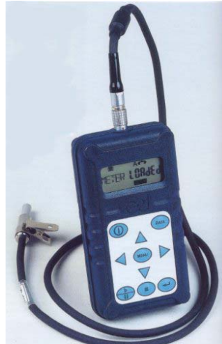
CEL-320 Noise dosimeter
