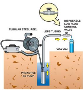
The Low Flow Control valve will allows the user to obtain 10 ML per minute
